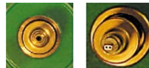
Fig.6 The older "pipe" type nozzle (left) and 0201 nozzle (right).
